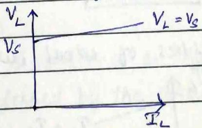
\* But practically every voltage source has small internal voltage resistance shown in series with voltage source and is represented by  $R_{se}$
