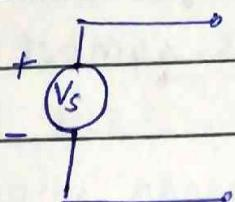
\* Ideal voltage source connected to the load.
