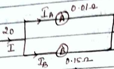
$$\text{using current division } I_A = I \times \frac{R_B}{R_A + R_B}$$
