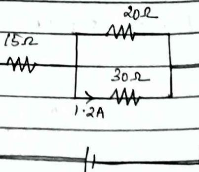
$$\text{Current in } 20\Omega \text{ is } V/R = 36/20 \\ = 1.8A$$
