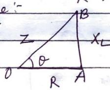
From the phasor diagram, we can separate the voltage triangle OAB. If each side of this triangle is divided by  $I$ , the result is the impedance triangle.
