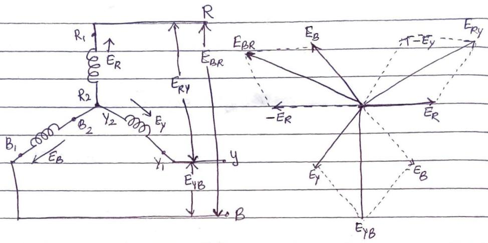
\* This system is obtained by joining together similar ends, either the start or the finish. The other ends are joined to the line wire.
