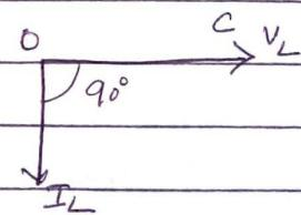
(c) Phasor diagram for L, rotated by 90°
