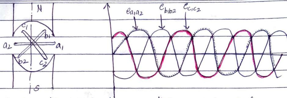
Accordingly, the instantaneous value of the emfs induced in the coil  $a_1, a_2, b_1, b_2$  and  $c_1, c_2$  may be given as
